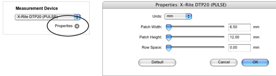
Figure 4.2. The Measurement Device Properties window can be used to create custom patch sets for the selected spectrophotometer.
